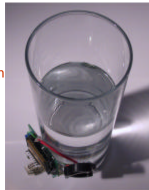
Objects contain pressure sensors for placement detection
