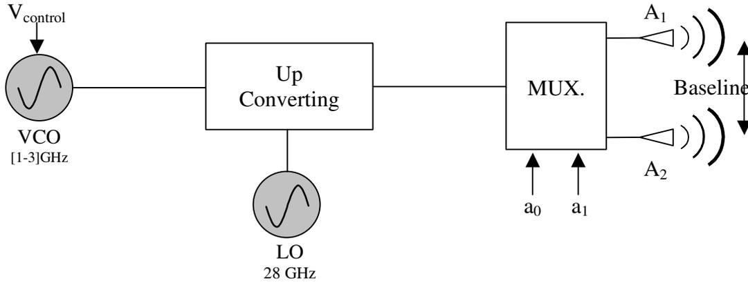
Fig. 2. : Schematic diagram of the dual transmitting principle
