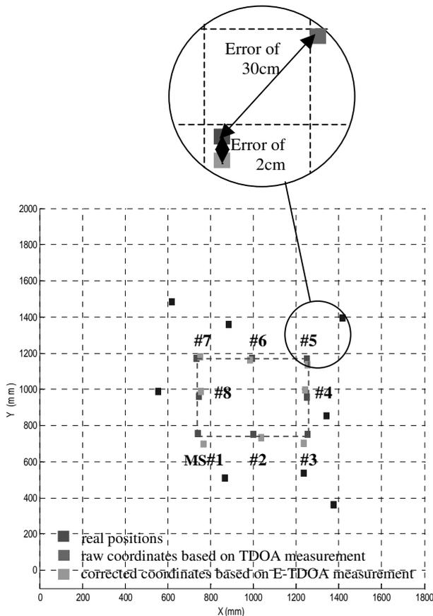
Fig. 6 : 8 mobile stations (MS) are located
